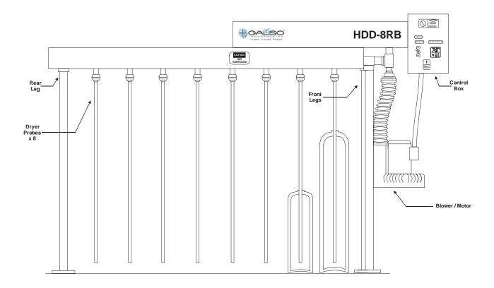
Figure 1, HDD Galiso Heavy Duty Dryer
