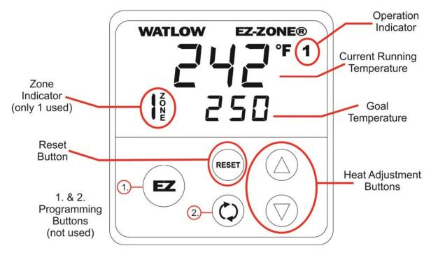
Figure 2, HDD Controller
